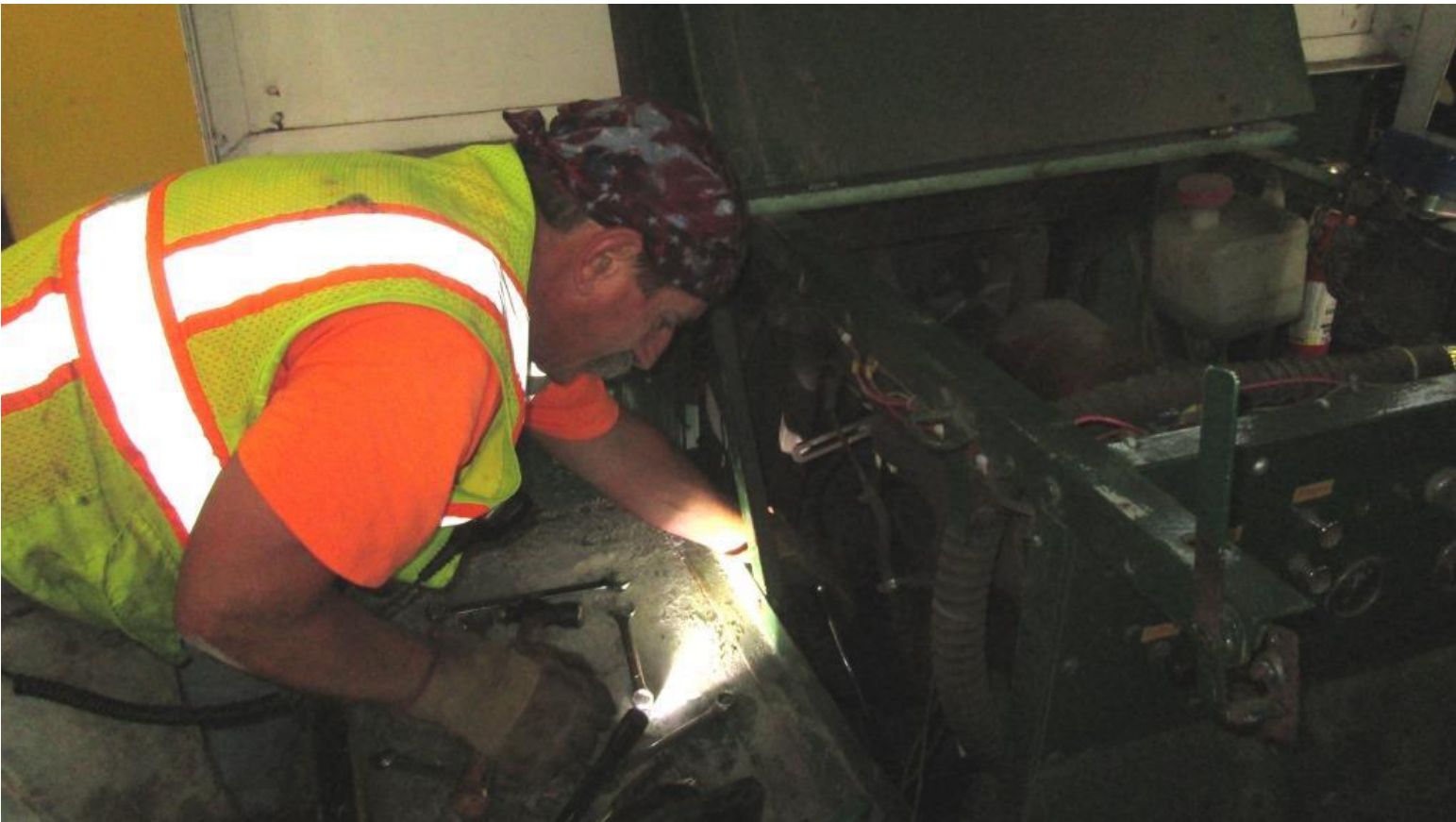
Joe replacing the A-4 motorcar's generator with an alternator
